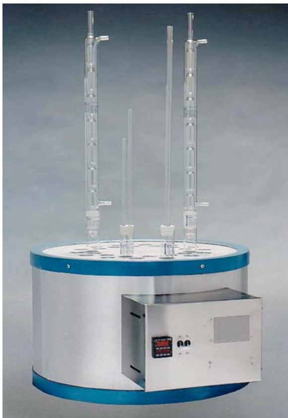
FIG. 1 A Typical Metal Block Type Ageing Oven
